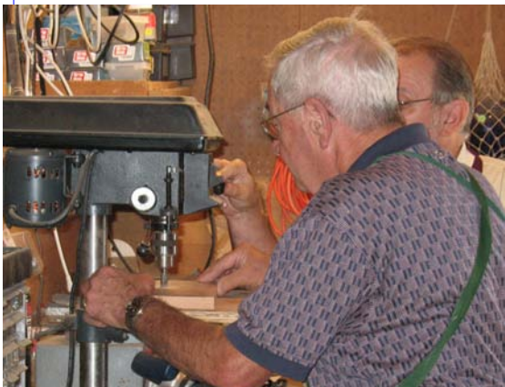
John S. and Pat use the drill press and rotary file to carve out the inset for the stone base
